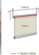
The Sheer-Suspension System offers an easy way to maximize the use and beauty of a Sheerhabitat fabric panel. This highly transparent combination of aluminum rod, clear nylon thread and adjustable hardware allow the panels to be displayed with clean lines and a solid construction.
