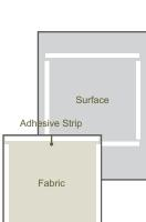
Sheer-Adhere Panels offer a simple way to attatch a fabric to walls, glass, cement and stone.
